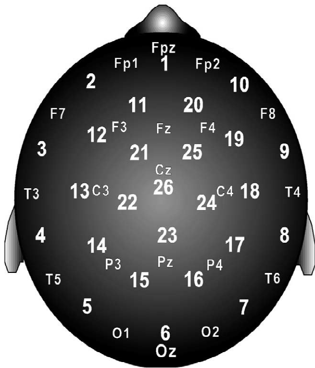
Fig. 2. Schematic of the electrode montage used for the ERP recordings. The montage is composed of 26 electrodes arranged in a quasi-geodesic configuration.
