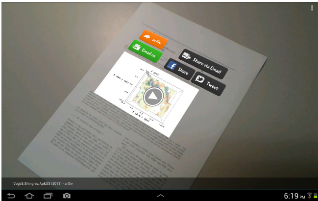
Fig. 10 Screen capture of the top of page 8 seen through the Layar app. Clicking the floating image overlaid over Figure 9 will start the animation. Additional buttons allowing the user to send us an email or share the article on social media are also included as additional examples of the wide variety of content that can be stored in a virtual layer of information.
