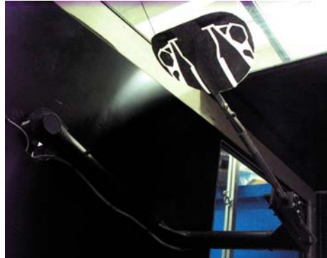
Figure 7-14. Wing topology optimized for minimum C_{L\alpha} built and tested in the wind tunnel.
