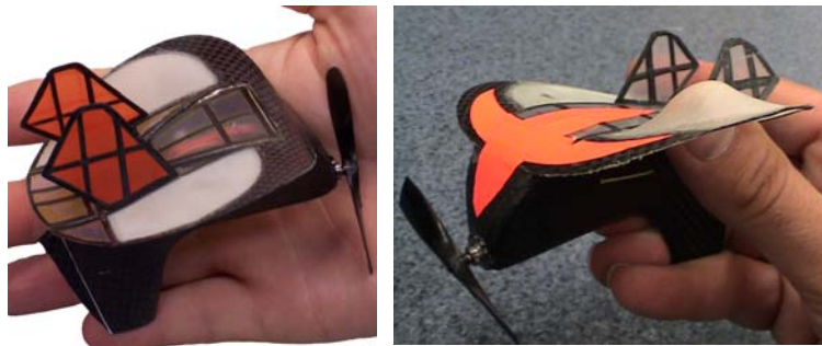
Figure 1-2. Perimeter-reinforced membrane wing design.
