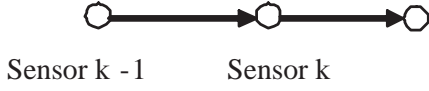
Fig. 1. Portion of a routing path where each sensor has only one upper stream sensor.
