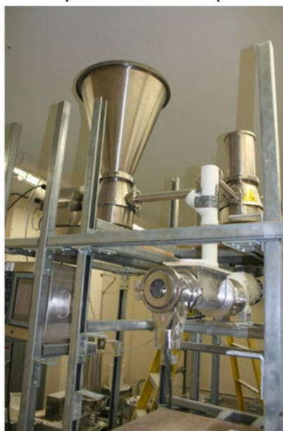
Gericke continuous mixer integrated with Schenck AccuRate LIW feeders
