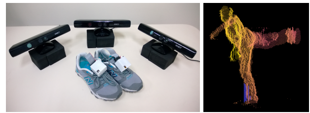
Figure 5: Data acquisition. (left) three Kinect cameras and a pair of pressure-sensing shoes; (right) input data to our motion capture system includes the point cloud obtained by three cameras and pressure data (blue lines) recorded by pressure sensors.
