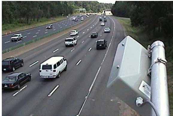
Figure 6 - Multi-lane highway monitoring using SAS-1
