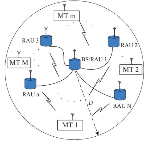
Fig. 1. Circular layout DAS configuration
