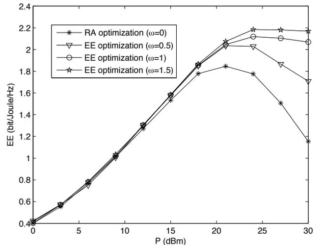
Fig. 3. EE versus total power of each RAU
