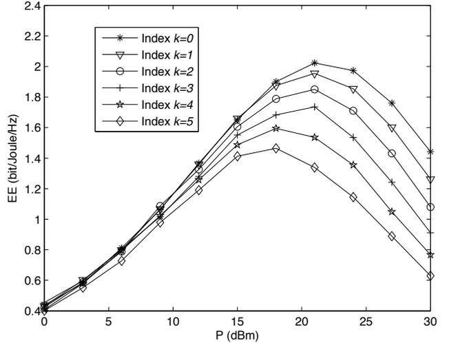
Fig. 7. EE versus different fairness indexes ( $\omega = 0.5$ )
