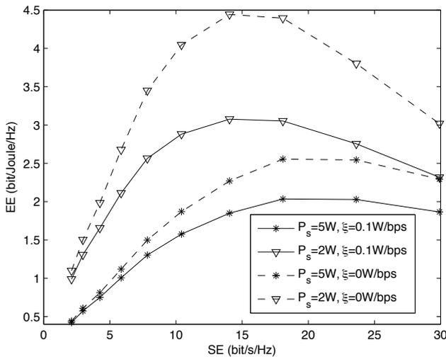
Fig. 5. EE versus SE under different circuit power parameters
