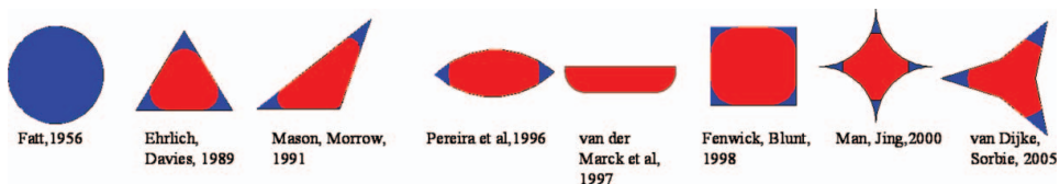
FIGURE 5. Various cross-sectional shapes used for pore throats in pore-network models (Color figure available online).
