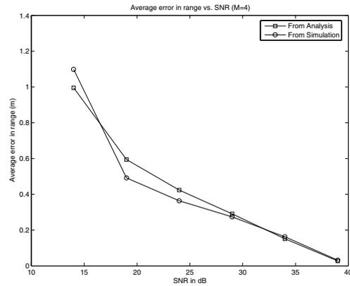
Fig. 5. Average estimation error in range vs. SNR ( $M = 4$ )
