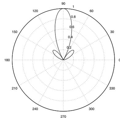
Fig. 2. A typical beam pattern for uniform linear antenna array ( $M=4$ )
