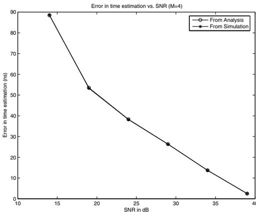
Fig. 4. Average estimation error in time vs. SNR ( $M = 4$ )
