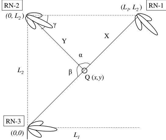
Fig. 1. Arrangement of three beacon nodes
