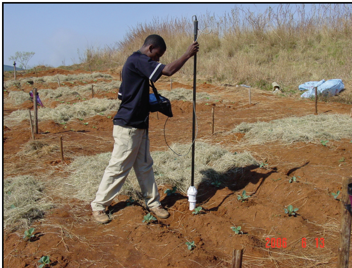
Figure 4.13 Student taking soil moisture readings with the Diviner 2000 at Ntembeni
