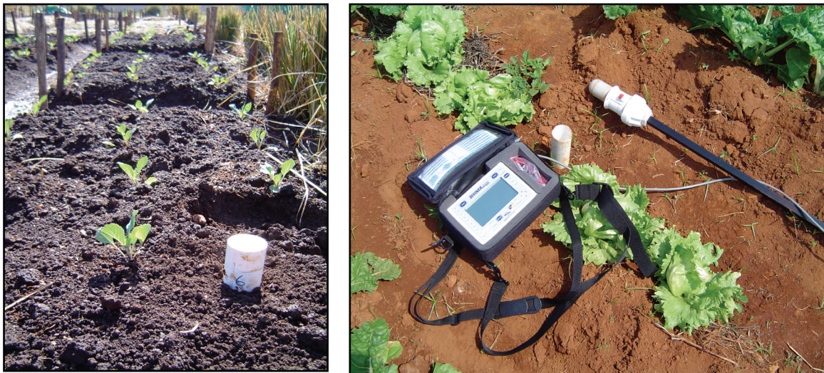
Figure 4.5 The Sentek Diviner 2000 system of soil water content measurement was used in this study. The left picture shows an access tube installed within a bed, whilst the right picture shows the Diviner 2000 instrument
