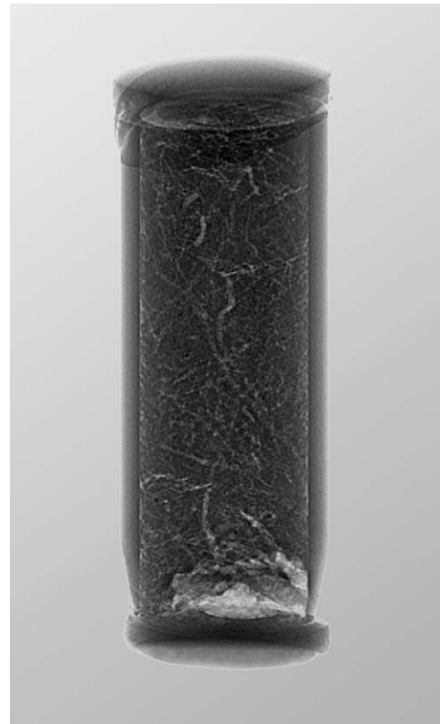
Fig. 3. X-ray tube CT-generated projection of the undisturbed soil (HL) cores used in this study.
