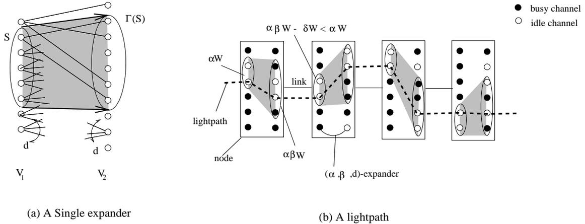
Figure 12: Using an expander for non-blocking networks.
