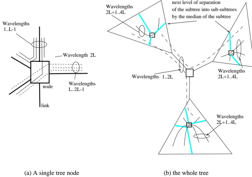
Figure 8: Dynamic allocation of wavelengths that go through a single tree node and the global picture of the tree
