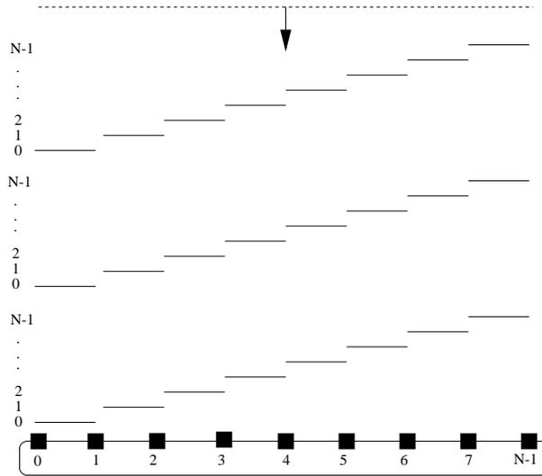
Figure 4: A worst case set of lightpaths for the Circular-First-Fit algorithm. The requests arrive starting from the bottom left request and proceeding in rows to the top right request.
