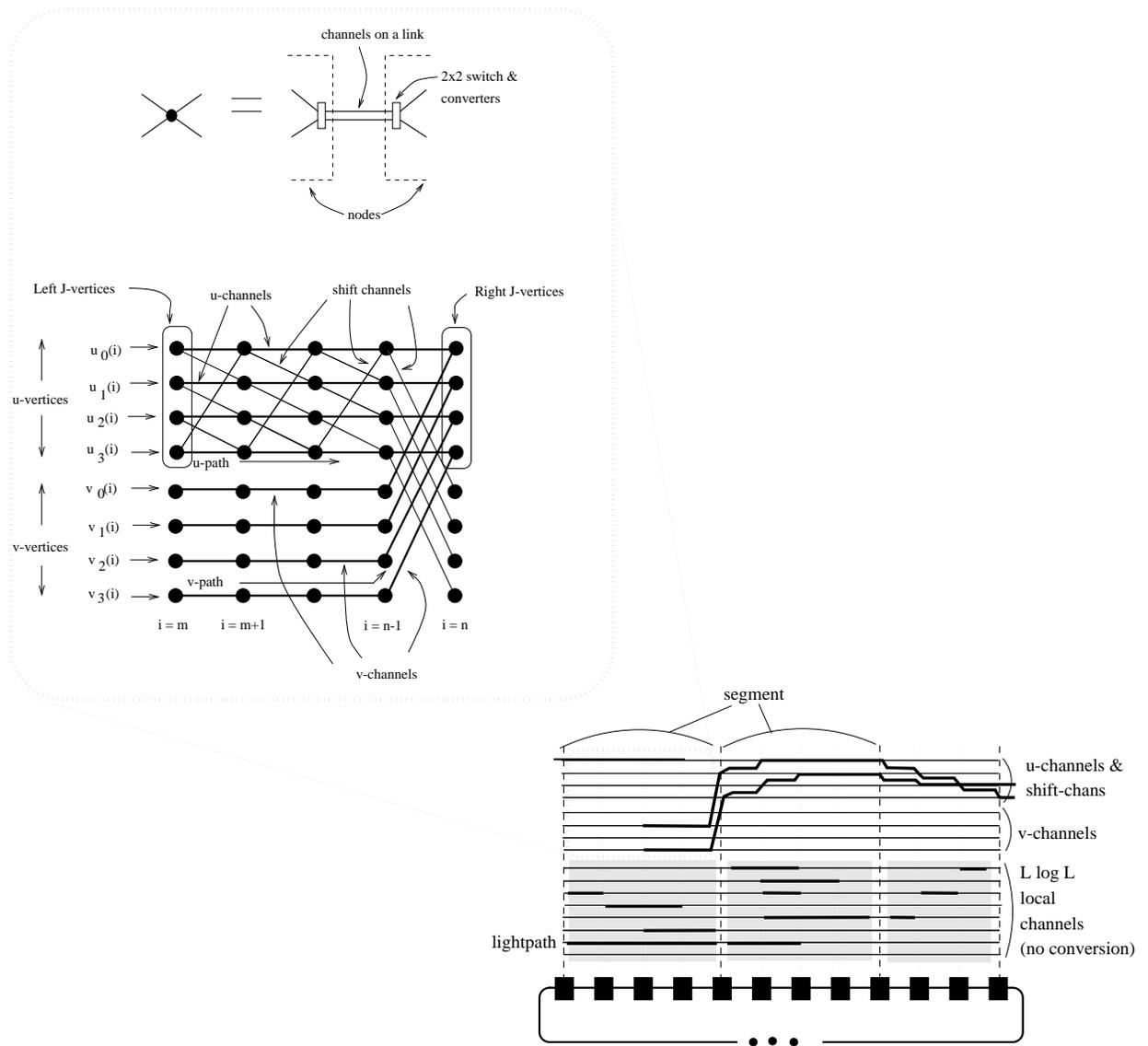
Figure 14: lightpath configuration in the proposed network and an enlarged subgraph of  $G^*$  corresponding to the segment of the ring with links  $\{m, m+1, \dots, n-1\}$ , and  $L = 4$ . The u-channels and v-channels are shown as thick lines, while the shift channels are shown as thin lines.
