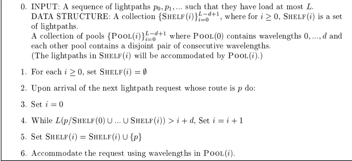
Figure 15: Incremental allocation of lightpath requests (IWLA)
