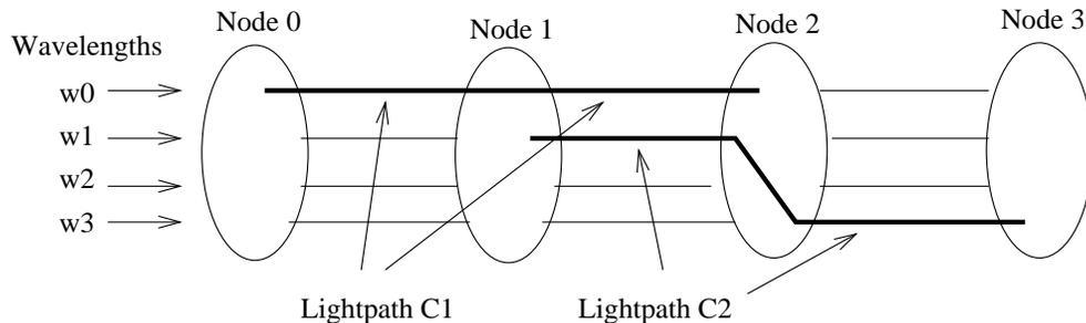
Figure 1: A WDM network with wavelengths  $\{\omega_0, \omega_1, \omega_2, \omega_3\}$  and two lightpaths  $C1$  and  $C2$ .
