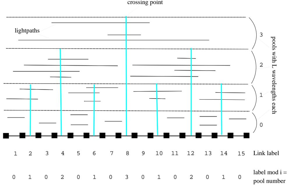
Figure 6:  $\log_2 N$  layers of  $L$  wavelengths each to accommodate the traffic pattern on a line, as in Figure 7.
