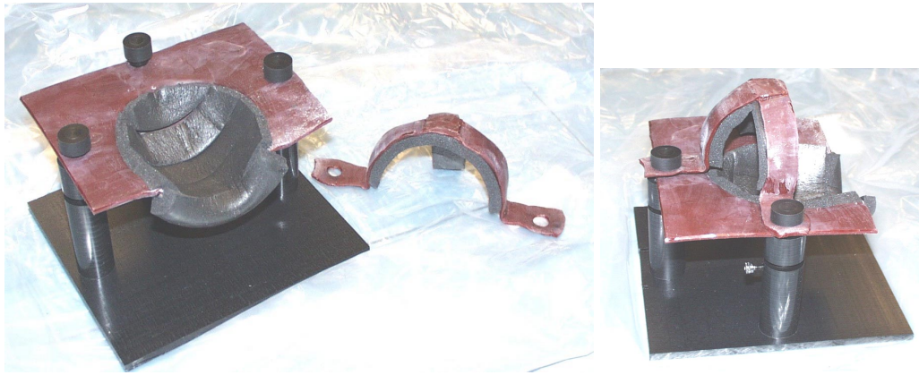
Figure 2.7.7 The first fibre holder, prior to the fibres being fitted.
