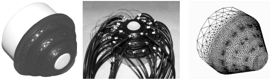
Figure 2.7.24 Conical breast fibre holder: three rings can be separated to create an annulus for various breast sizes. (right) the FEM mesh generated to allow the conical shape of the phantoms or the breast to be modelled.
