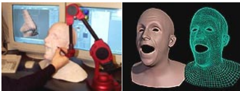
Figure 2.9.21 Microscribe 3D co-ordinate recording arm used to map the surface of a head. From: Immersion Medical, 55 West Watkins Mill Rd, Gaithersburg, Maryland 20878 USA, Telephone: 301.984.3706, Fax: 301.984.2104, http://www.immersion.com/products/3d/overview.shtml . Graphics from: http://www.rsi.gmbh.de/ms-max_e.htm
