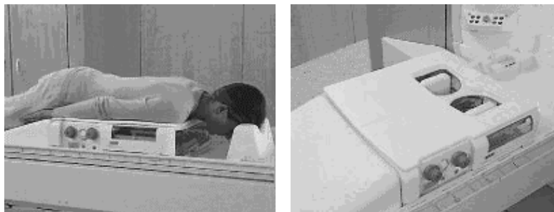
Figure 2.9.24 Acquiring and MRI of the breast requires the subject to lie prone on the bed with the breasts hanging into holes which house RF coils.
