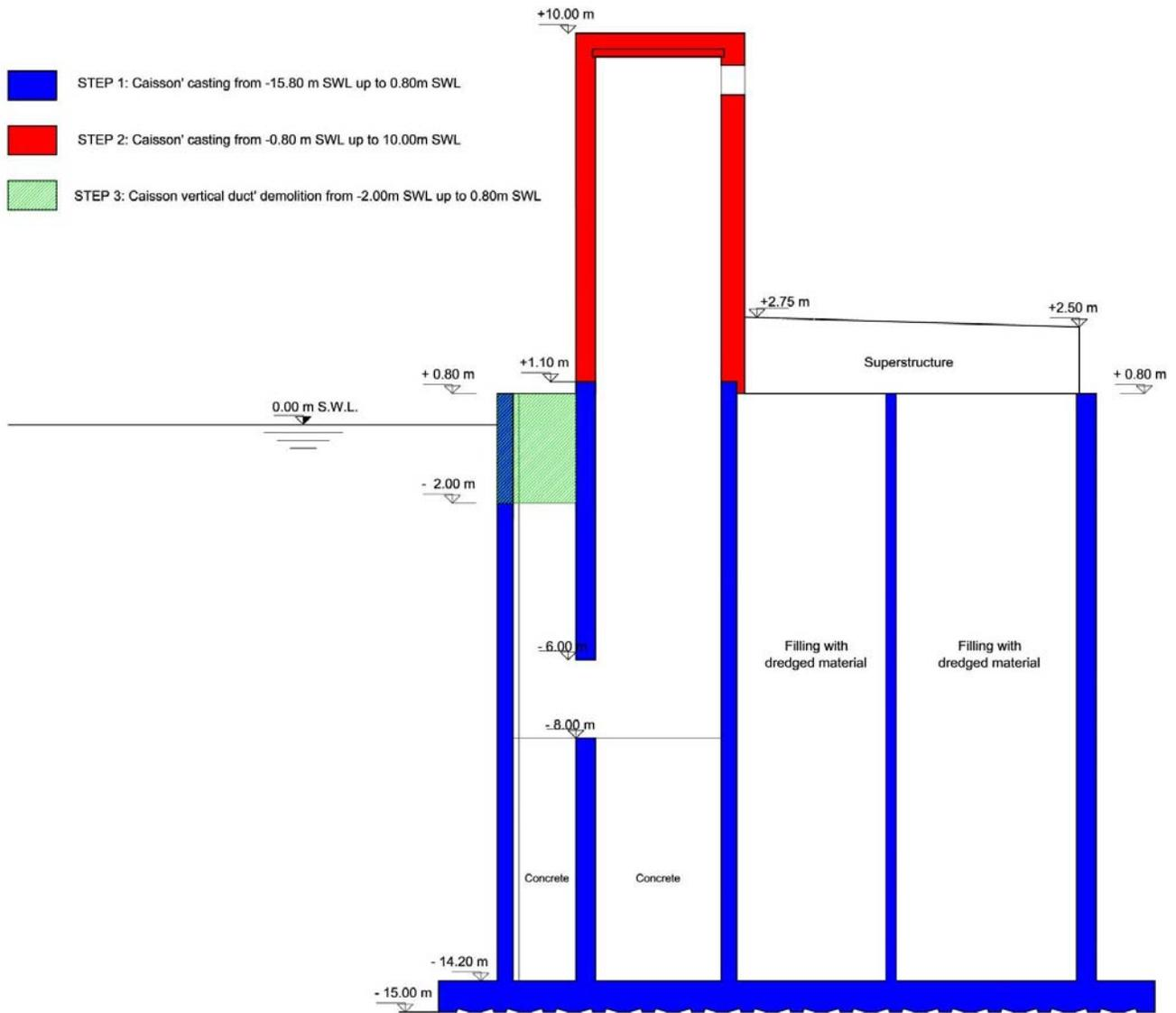
**Figure 8.** Reference frame of the REWEC3 caisson.
