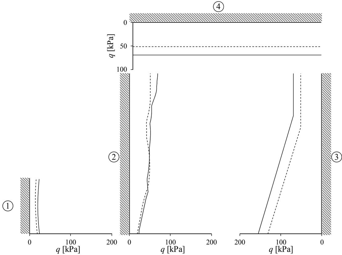
**Figure 3.** Loads on the walls of the REWEC3. The numbering denotes: sea side wall of the U-duct (1); sea side wall of the inner chamber (2); land side wall of the inner chamber (3); upper wall (4). It has been assumed:  $H_S = 5\text{m}$  (dotted line);  $H_S = 6\text{m}$  (continuous line).
