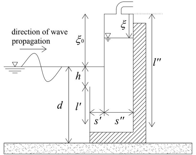
Figure 1. Reference sketch of the REWEC3 plant.
