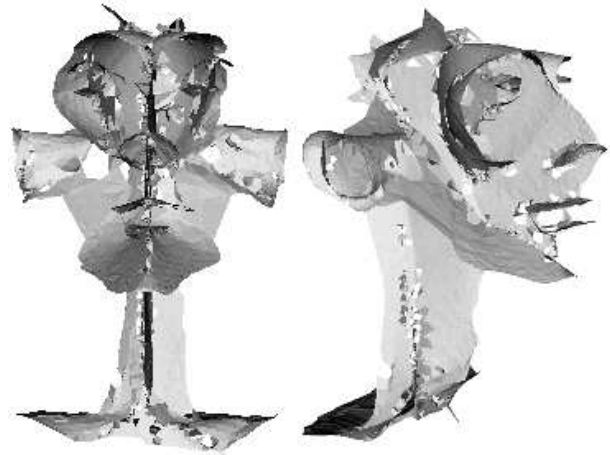
Fig. 7. Reconstruction of inner skeleton of Mannequin head model by Crust algorithm. Note many holes near non-manifold skeleton on points.
