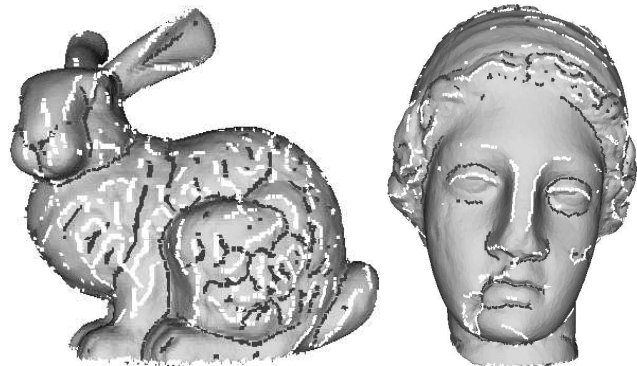
Fig. 19. Salient ridges (white) and ravines (black) detected on complex polygonal models.
