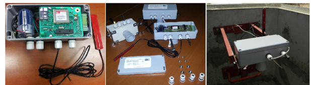
Fig. 2: Photographs of the developed smart water meter.
