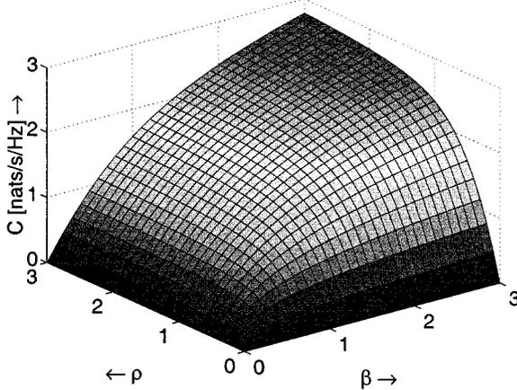
Fig. 5. Channel capacity of the antenna-array channel per unit number of receive antennas with  $10 \log_{10}(P/\sigma^2) = 9$  dB.
