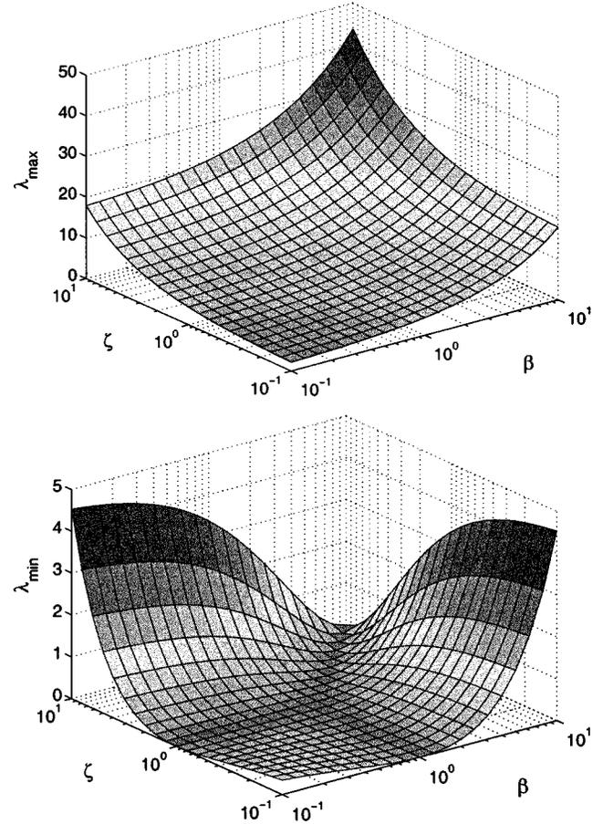
Fig. 2. Largest and smallest (nonzero) eigenvalue of  $\mathbf{C}$  as a function of the two loads  $\beta$  and  $\zeta$  in the asymptotic limit.
