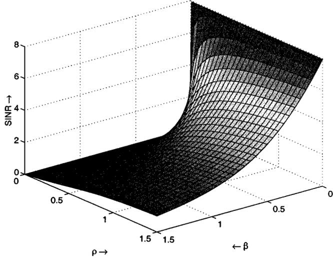
Fig. 3. SINR as function of system load  $\beta$  and richness  $\rho$  for  $10 \log_{10}(P/\sigma^2) = 9$  dB.
