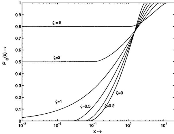
Fig. 1. Asymptotic eigenvalue distribution for system load  $\beta = 0.5$  and various channel loads.
