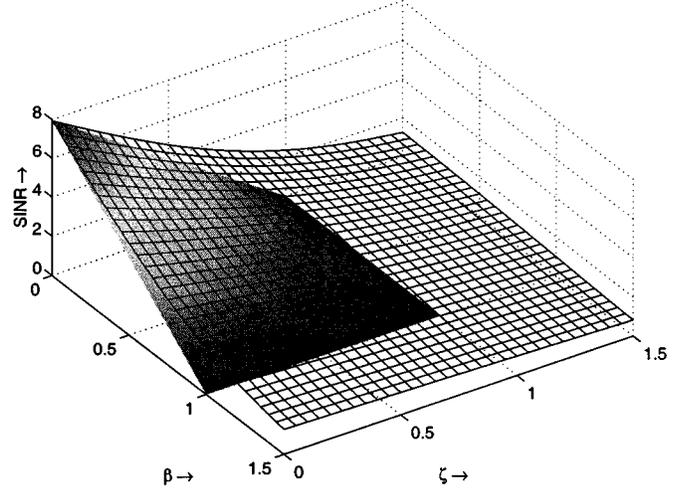
Fig. 4. SINRs of nulling (shaded) and optimum beam forming for  $10 \log_{10}(P/\sigma^2) = 9$  dB.
