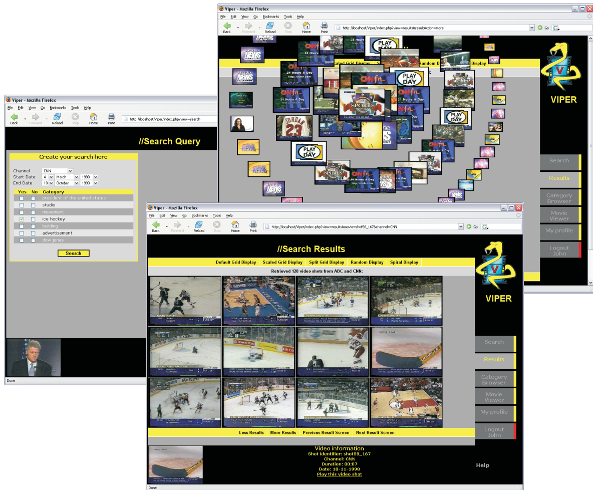
Figure 7.4: User interface of the Viper search engine. The left panel shows the search interface, the top panel shows a spiral visualization of a search on graphics and the bottom panel shows a grid visualization of ice hockey .
