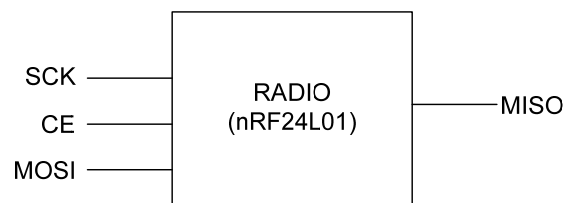
Figure 3. Radio SPI: inputs and outputs
