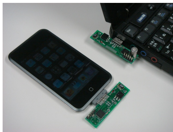
Figure 1. Appearance of “Parasitic Ambient Logger” System. (sensor modules attached to an iPod touch and a laptop computer)
