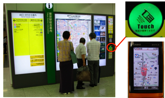
Figure 1. The NaviTa system at Tokyo Station. People can fetch a local map and store/service directory by touching their RFID-chipped mobile phones on the green “touch area.”
