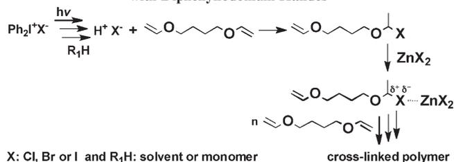
**Scheme 25.** Cationic Polymerization of Vinyl Ethers Initiated by Photolysis of Vinyl Halides in the Presence of Zinc Iodide
