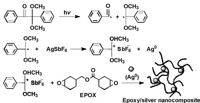
approach nanoparticle formation and UV cross-linking process were accomplished in one pot by simply irradiating appropriate formulations, obtaining the homogeneous distribution of the nanoparticles within the polymer network without any macroscopic agglomeration. Silver or gold nanoparticles and initiating species were formed in a single redox process. The overall strategy is represented in Scheme 31.
