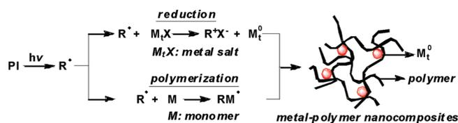
**Scheme 32. Synthesis of Metal–Polymer Nanocomposites by Cationic Polymerization**
