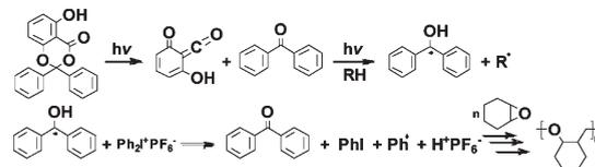
**Scheme 17.** 3,5-Diphenyldithieno[3,2-*b*:2,3-*d*]thiophene as Sensitizer for Iodonium Salt Decomposition via Electron Transfer To Generate Photoacids
