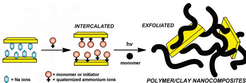
This methodology was further extended to indirect photoinitiating systems using free radical sources and photosensitizers.<sup>181</sup> In this connection it should be pointed out that in these systems the photochemical step is involved only in the generation of reactive species, and the propagation proceeds by a thermal reaction.
