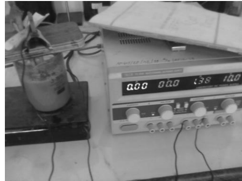
Fig-1: Bench-scale EC reactor with monopolar electrodes
