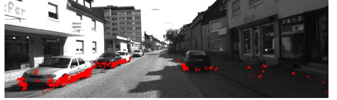
Fig. 3. Points labeled as obstacles using normal vectors
