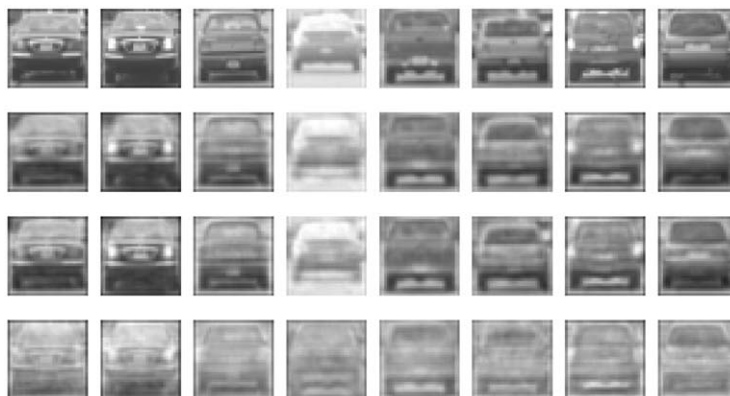
Fig. 8. Reconstructed images using the selected eigenvectors (first row): original images; (second row): using the top 50 eigenvectors; (third row): using the eigenvectors selected by SFBS; (fourth row): using the eigenvectors selected by GAs.
