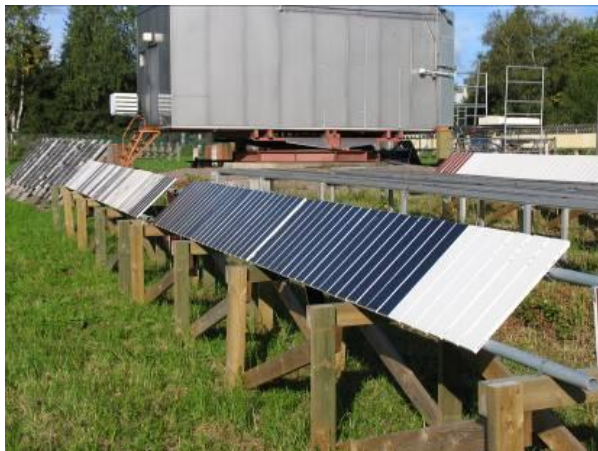
Figure 2. Outdoor test systems for coated plywood products at VTT Otaniemi.
