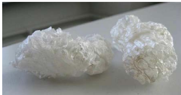
Figure 3. Plasticised starch foamed with water in an extruder.
