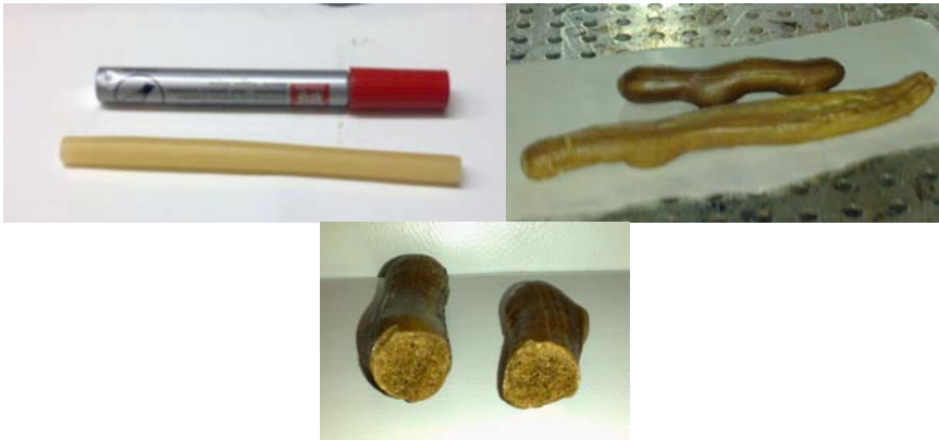
Figure 2. Starch compound (i) after extrusion, (ii) expansion in an oven, and (iii) expanded starch.
