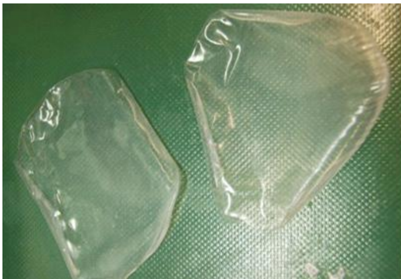
Figure 2. Cellulose films precipitated with a combination coagulant contained some 1:1 of (\text{NH}_4)_2\text{SO}_4 and \text{Na}_2\text{SO}_4 in dilute \text{H}_2\text{SO}_4 .
