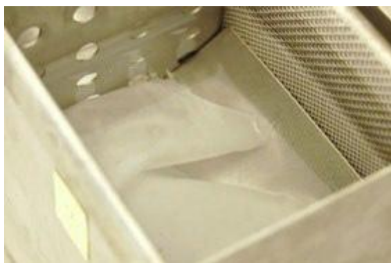
Figure 1. Film precipitated from 6 g of starch solution containing 4:1 of KOH and NaOH.
