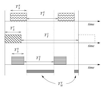
Fig. 3. The effective time available for transmission  $T_a^y$  for the CR user y.
