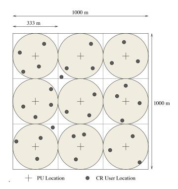
Fig. 5. Topology used for performance evaluation
