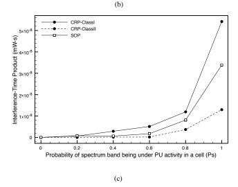
Fig. 8. The effect on the PU receivers due to transmissions of the CR users on the chosen route
