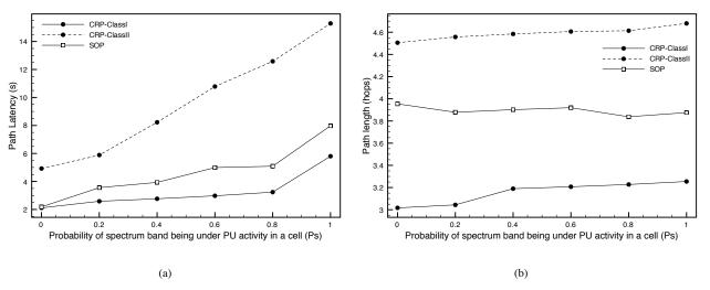
Fig. 6. The end-to-end path latency (a) and the path length (b) are shown for varying probability of spectrum band being under PU activity in a cell (Ps).
