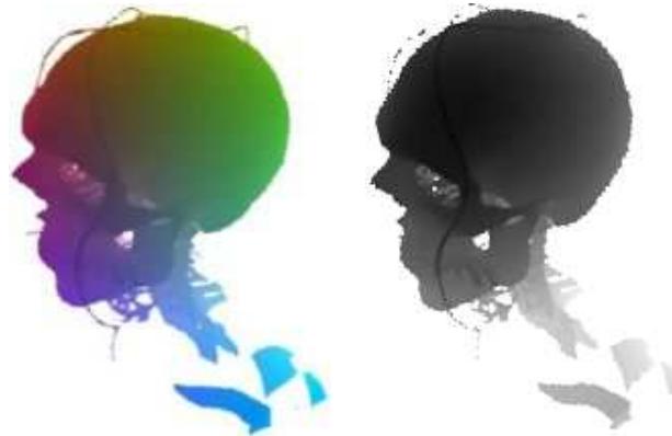
Figure 4.2: The first hit points in color-coded volume coordinates as seen from the light source (left) and the resulting depth map (right). Both maps have a resolution of 512 \times 512 texel and are generated during rendering the visible human head data set (see Figure 4.7).
