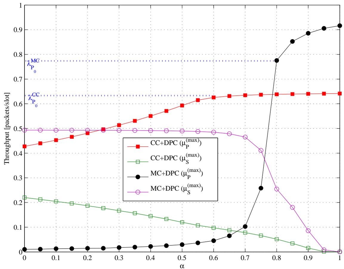
Fig. 4. Maximum throughput for primary and cognitive user versus  $\alpha$  for CC+DPC and MC+DPC;  $R_0 = 2$  BPCU,  $K = 2$  cognitive users,  $d = 0.6$ ,  $P_0 = 6$  dB.
