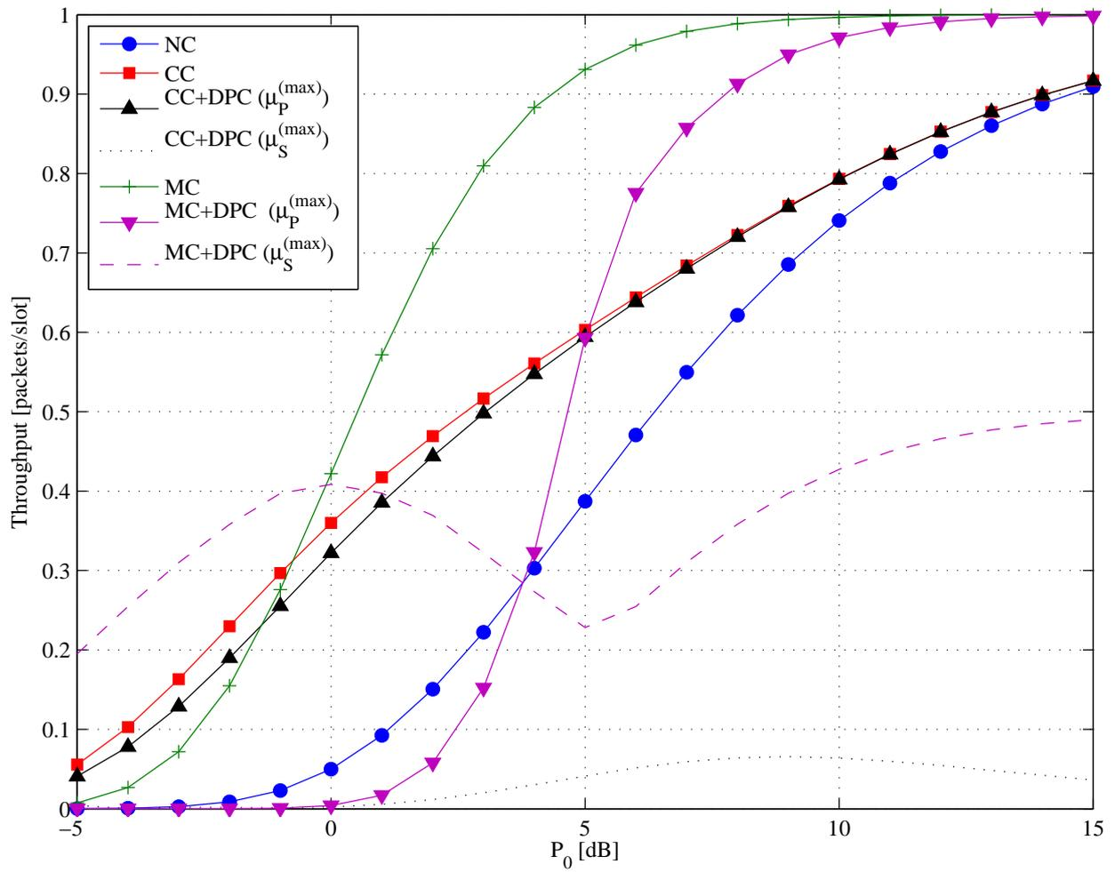
Fig. 6. Maximum throughput for primary and cognitive user versus the SNR of the direct link;  $R_0 = 2$  BPCU,  $K = 2$  cognitive users,  $d = 0.6$  and  $\alpha = 0.8$
