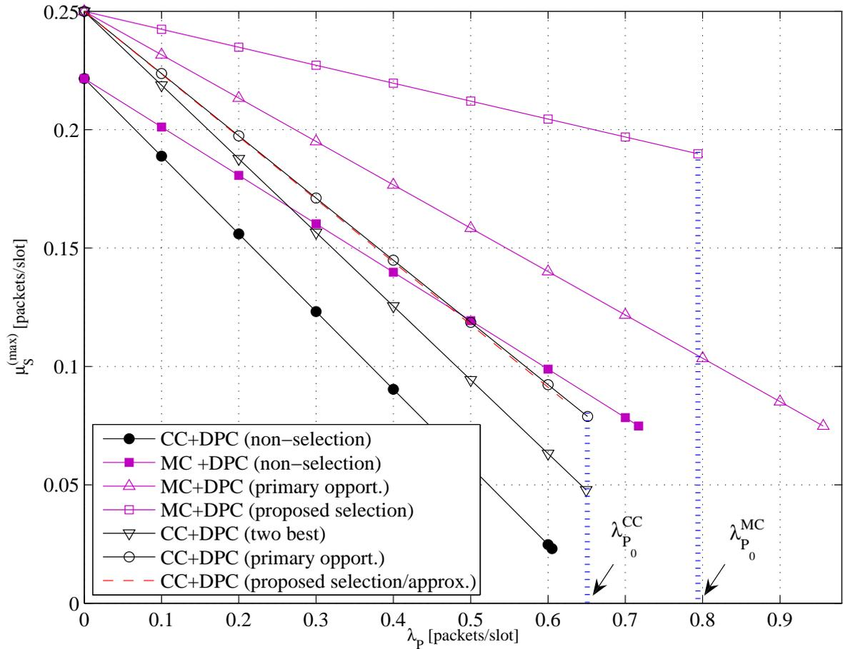
Fig. 8. Maximum throughput  $\mu_S$  versus  $\lambda_P$  for DPC schemes for different selection criteria: non-selection, primary based selection (two best), proposed selection;  $K = 4$ ;  $R_0 = 2$  BPCU,  $d = 0.6$ ,  $P_0 = 6$  dB,  $\alpha^{CC} = 0.6$  and  $\alpha^{MC} = 0.8$ .
