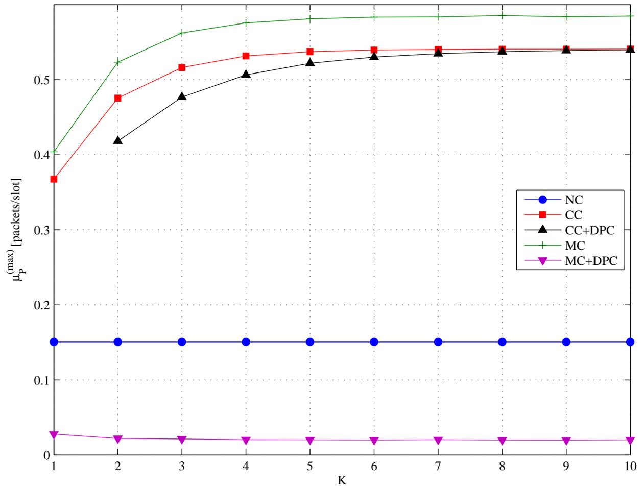
Fig. 7. Maximum throughput for primary user versus  $K$ ;  $R_0 = 2$  BPCU,  $d = 0.5$ ,  $P_0 = 2$  dB and  $\alpha = 0.8$ .
