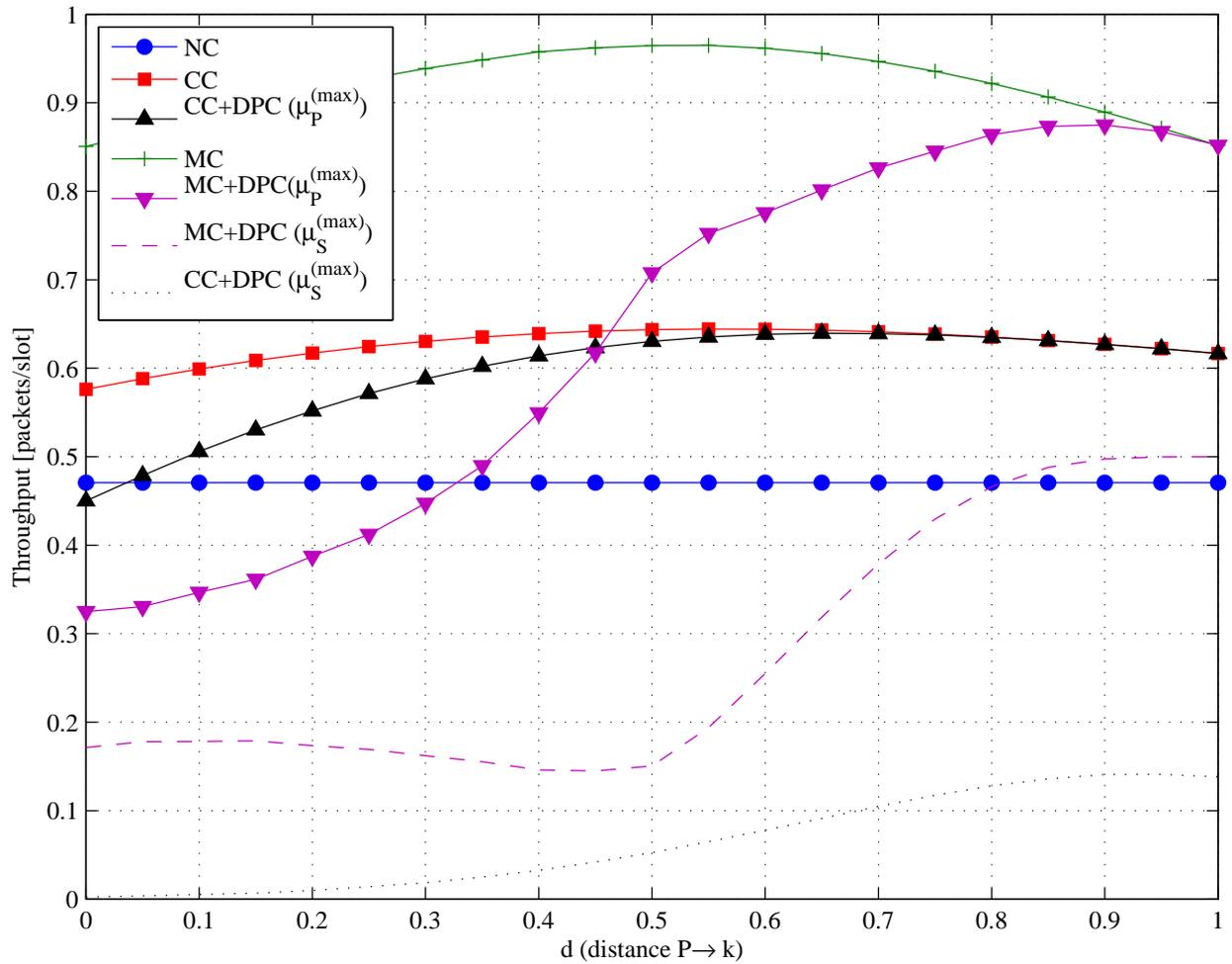
Fig. 5. Maximum throughput for primary and cognitive user versus the distance between primary user and cluster;  $R_0 = 2$  BPCU,  $K = 2$  cognitive users,  $P_0 = 6$  dB,  $\alpha^{\text{CC}} = 0.7$  and  $\alpha^{\text{MC}} = 0.8$ .
