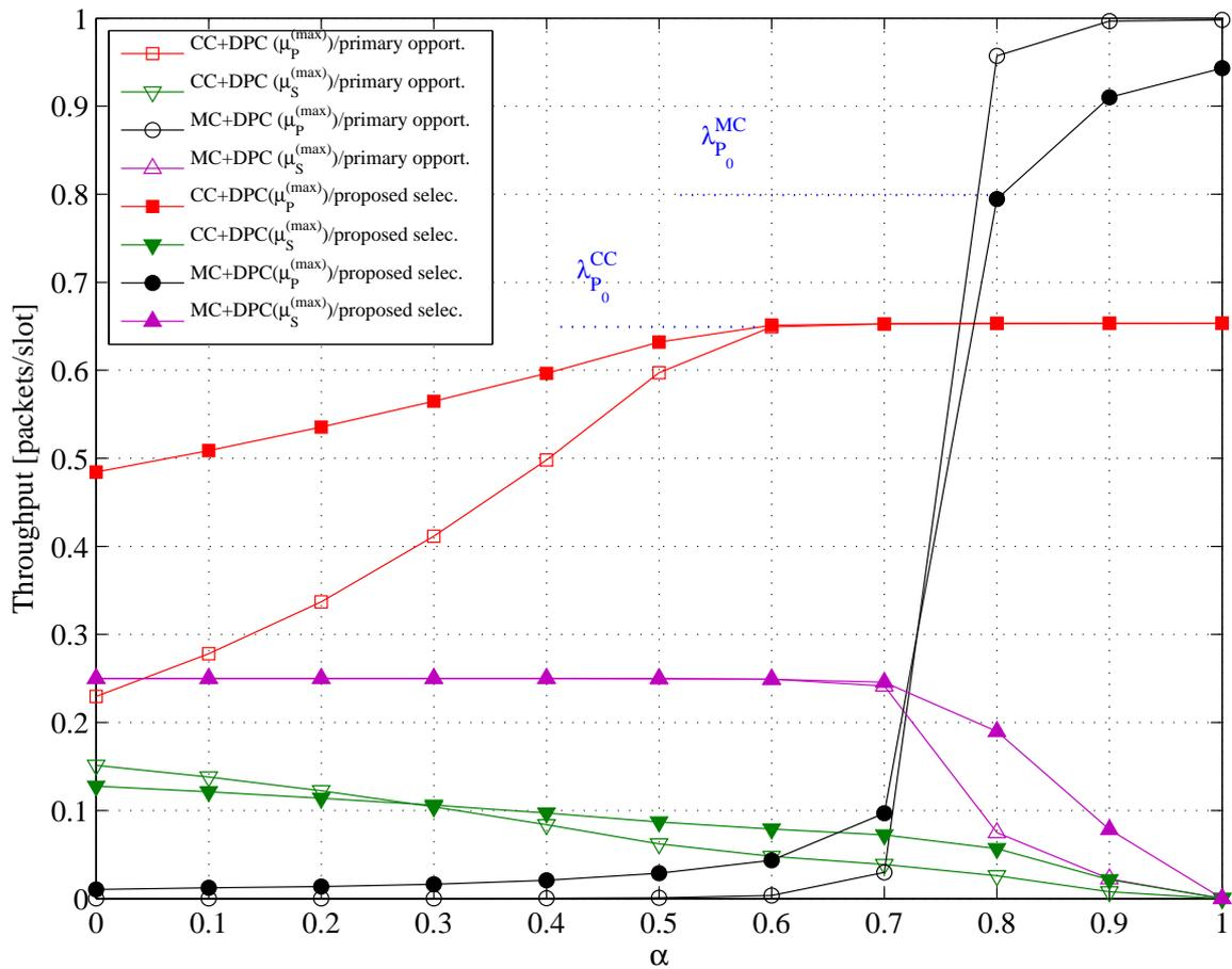
Fig. 9. Relay selection for DPC-based schemes versus the parameter  $\alpha$ ;  $K = 4$ ;  $R_0 = 2$  BPCU,  $d = 0.6$ ,  $P_0 = 6$  dB.
