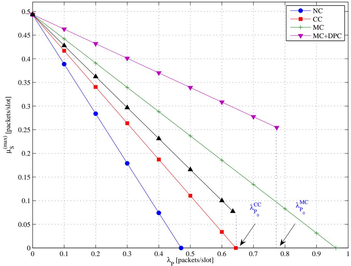
Fig. 3. Maximum throughput  $\mu_S$  versus  $\lambda_P$  for NC, CC, CC+DPC, MC, and MC+DPC;  $R_0 = 2$  BPCU,  $K = 2$  cognitive users,  $d = 0.6$ ,  $P_0 = 6$  dB,  $\alpha^{CC} = 0.7$ ,  $\alpha^{MC} = 0.8$ .
