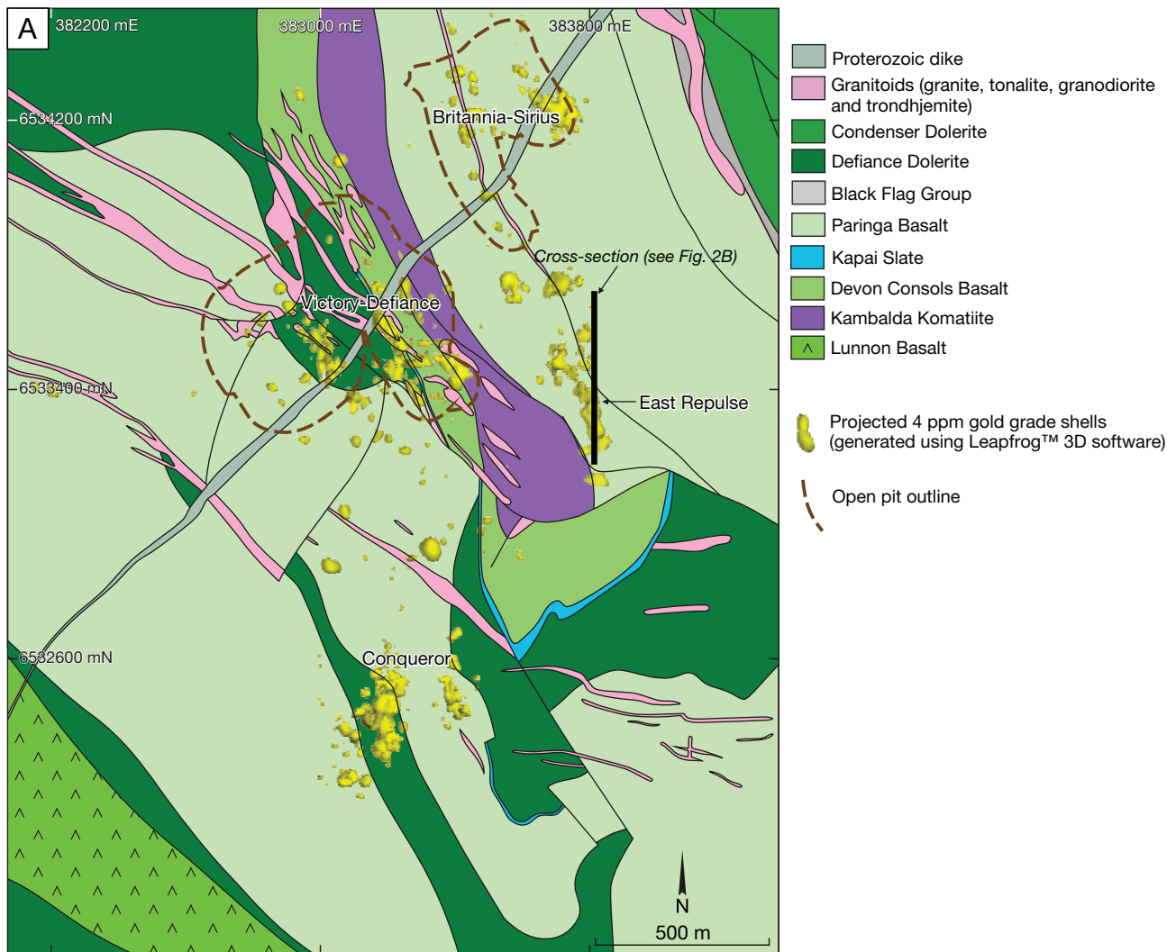
FIG. 2. A. Geologic map of the area surrounding the East Repulse deposit, showing the location of major gold deposits, as well as the location of the studied cross section shown in (B) (modified from Watchorn, 1998). B. A south-north geologic cross section of the East Repulse deposit. Samples analyzed in this study were collected from diamond drill holes along this section.
