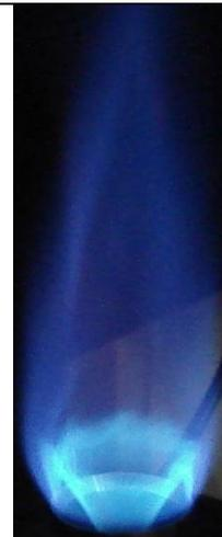
Figure 4(b): Photo of flame just before flashback through outer wall boundary layer,  $S_{II}=1.04$
