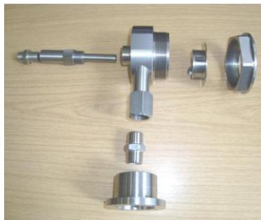
Figure1: Exploded view of Swirl Burner
