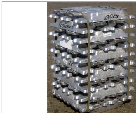
Figure 3(a): Traditional foundry ingot
