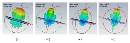
Fig. 5. 3D-polar plot of beam shape radiation patterns by turning ON the EBRS (a) switch i (b) switches i and ii (c) switches i, ii, and iii (d) switches i, ii, iii, iv and v
