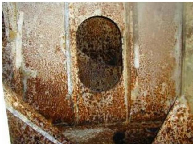
**Fig. 21: Corrosion in ballast tank due to insufficient protection**
