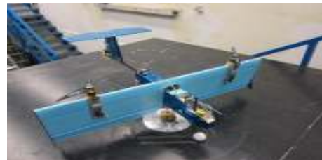
Fig. 10. Tiltwing VSTOL validation aircraft in vertical take-off configuration
