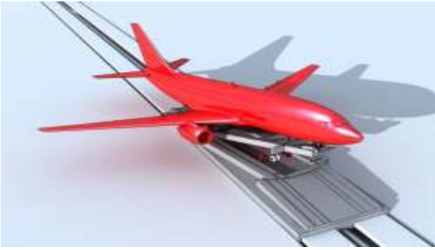
Fig. 1. Landing and take-off without landing gear and use ground-based MAGLEV power.
