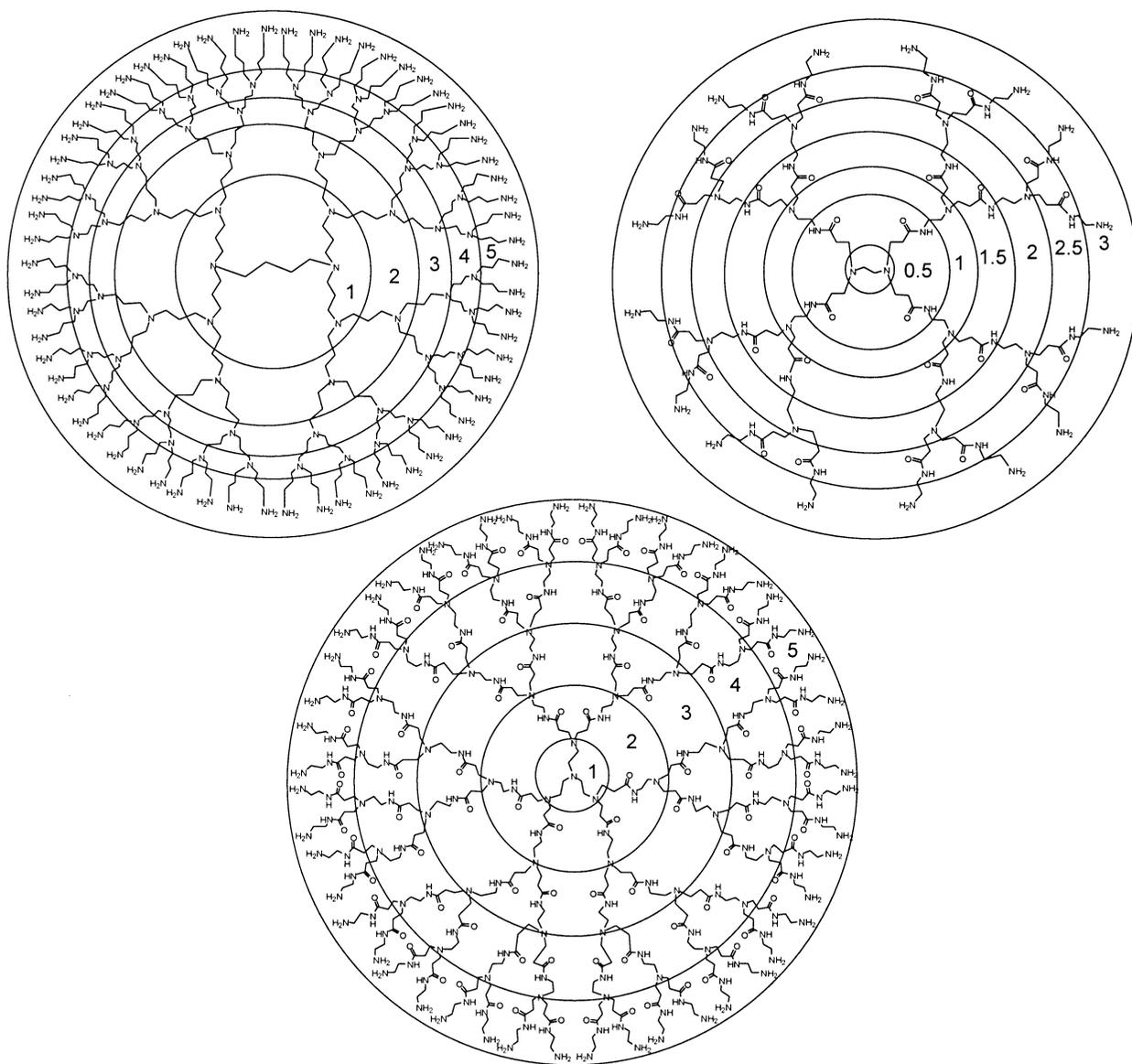
**Fig. 1** Common commercially available dendrimers. Top left: Polypropylene imine dendrimer (G5). Top right: Polyamido amine dendrimer (G3). Bottom: Polyamido amine (Starburst™) dendrimer (G5). Each generation is marked with a circle.
