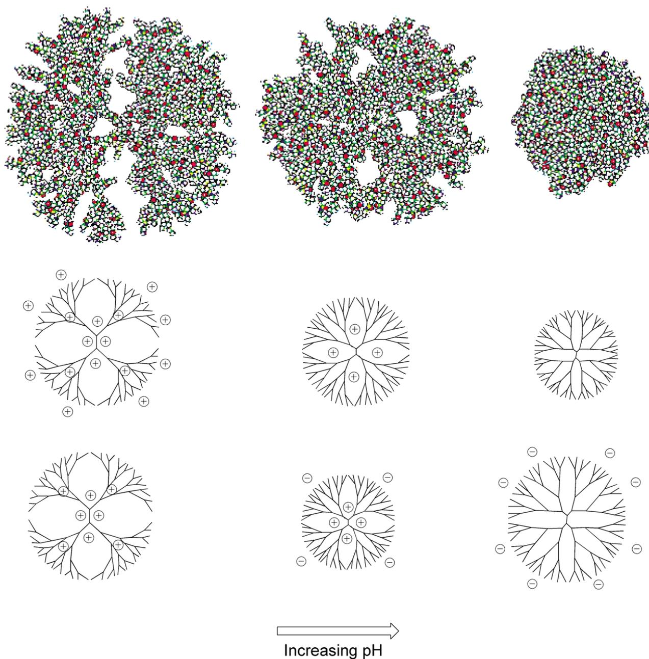
**Fig. 5** Top row: Three dimensional depiction of conformational change of an amino-terminated PAMAM dendrimer at increasing pH (reprinted with kind permission from reference 28, copyright (2002) American Chemical Society). Middle row: Two-dimensional depiction of the conformational change of an amino-terminated PAMAM dendrimer upon increasing pH. Bottom row: Two-dimensional depiction of the conformational change of a carboxy-terminated PPI dendrimer at increasing pH.<sup>30</sup>
