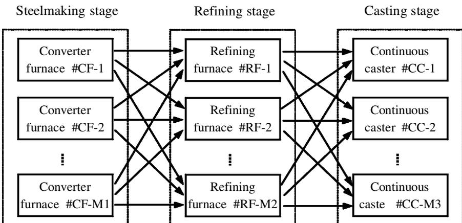
Figure 1. The steelmaking process.
