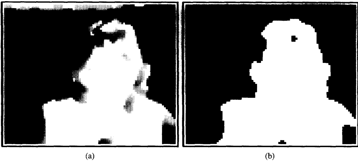
Fig. 4. Dynamic segmentation images obtained using past and present change detection masks: (a) sequentially fused images of Miss America sequence of frames 70 to 90; (b) the resulting candidate regions for the silhouette of Miss America in frame 90.
