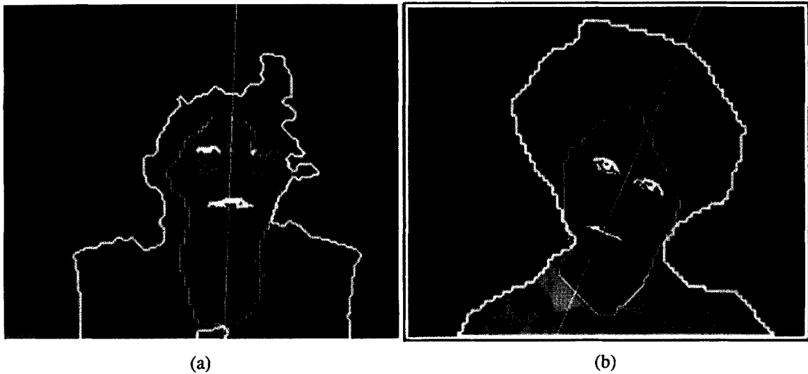
Fig. 13. Selected regions representing the features of interest (silhouette, face, eyes and mouth) and the corresponding eye vertical for (a) frame 79 of the Miss America sequence, and (b) frame 205 of the Talking sequence.
