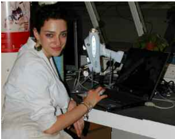
Figure 2: Molly Zuckerman using handheld X-Ray Florescence Spectrometry to measure levels of mercury in human bone from seventeenth-century London skeletal samples, Museum of London's Centre for Human Bioarchaeology Laboratory. This technique allows nondestructive analysis of the elements contained within various materials, including human bone (Photo credit: Lilly Zuckerman).
