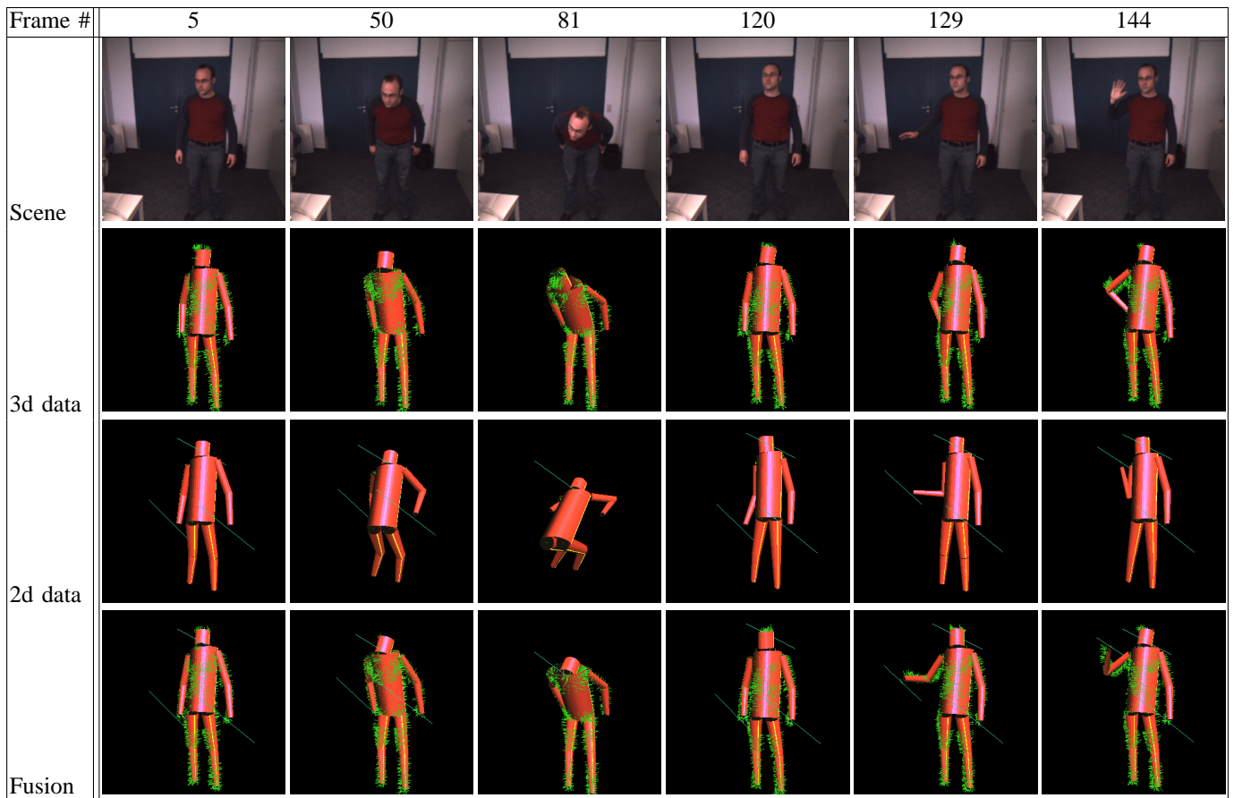
Fig. 4. Experiments with different sensor inputs, taken from a sequence containing a “bow” and a “wave” movement. The frame number is displayed on the top. The used 2d and 3d correspondences have been added to the resulting model images.
