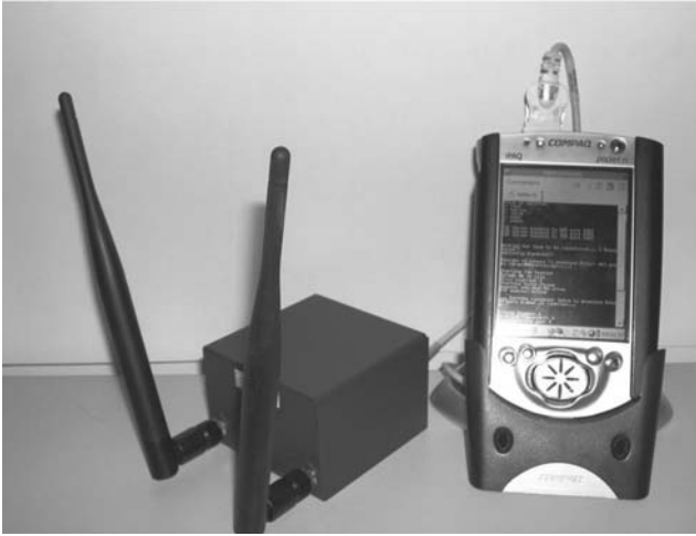
Figure 15.2 A 4G Access Cube on the left (mesh device), connected via Ethernet to a PDA (processor unit)
