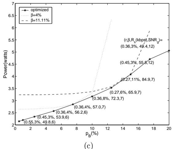
Fig. 3. Power minimization for a wireless communication system.
