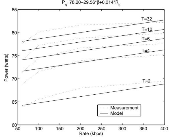
Fig. 2. Power consumption for coding "foreman.qcif", with a software implementation of the H.263 coder running on an IBM thinkpad with a 360 MHz Pentium II processor.
