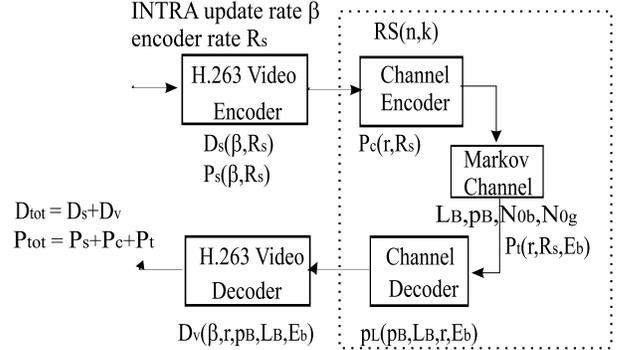
Fig. 1. The wireless communication system considered in this paper.
