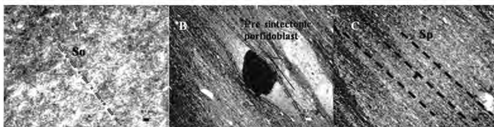
Figure 3. Micrographs of some thin sections on fine-grained slate from the upper sequence (PF1) of the Luearca Formation: A, C, PPL (x 2.5); B, XPL (x 2.5). AFM diagram plot of the study sample (Luearca Slate, Jola quarry). Samples from other sites of the Truchas domain (Casaio and Rozadais formations) and from the Schist-greywacke Complex (South Central-Iberian Zone) are shown for comparison. Mineral and pelite compositional fields taken from Pattison (2001) and Miyashiro (1994).
