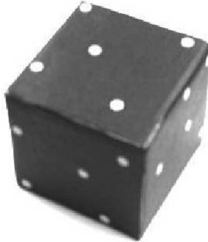
Figure 2.4: Cube with projective invariant retro-reflective infrared markers.
