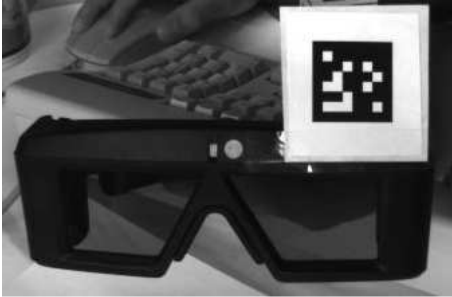
Figure 4.4: Pair of shutter glasses equipped with a marker for head tracking.
