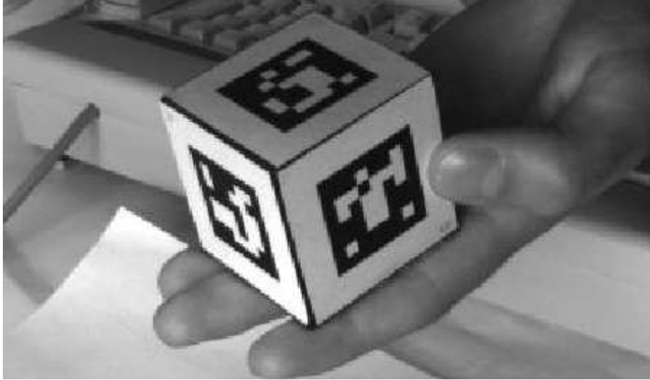
Figure 4.5: Cube device with a marker on each side. The cube is chosen because it always has at least one visible side in the camera image independent of the orientation.
