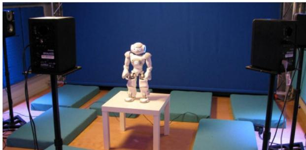
Figure 2: NAO in the sound-localisation experiment setup
