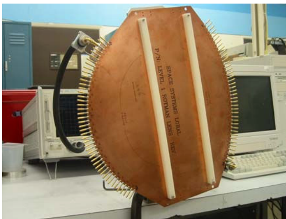
Fig. 16 Network analyzer measurement of prototype lens.
