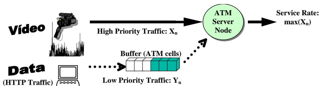
Figure 4. Proposed scheme for loss measurement of low priority traffic.
