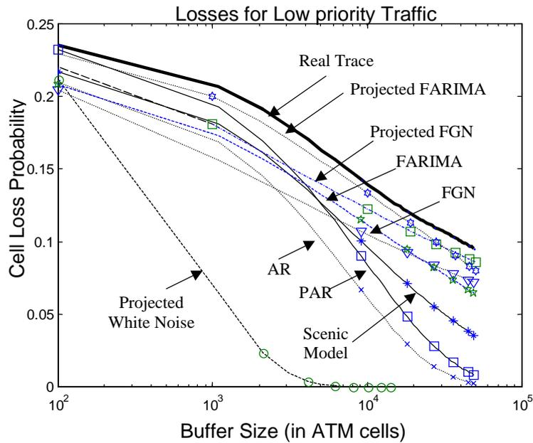
Figure 5. Losses for low priority traffic (HTTP flow)
