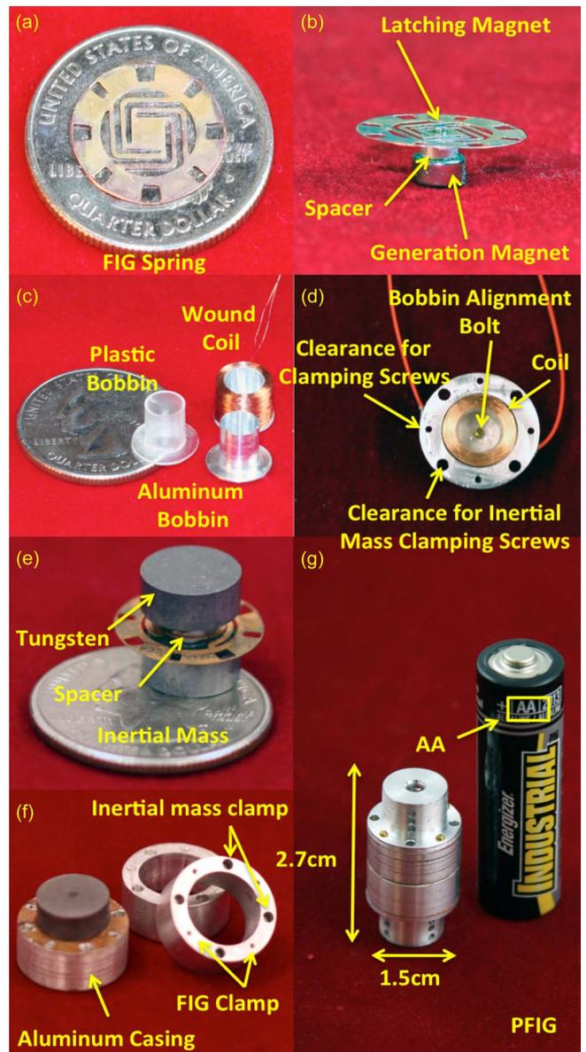
Fig. 11. Photographs of fabricated PFIG components and completed generator. (a) FIG spring on top of U.S. quarter. (b) FIG spring assembly. (c) Machined bobbins on top of a U.S. quarter and wound coil. (d) Assembled FIG casing with a coil fixed inside. (e) Inertial mass assembly. (f) Inertial mass inside a partially opened casing. (g) Completed PFIG alongside a standard AA battery.
