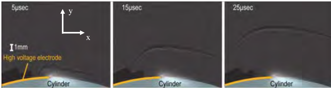
Figure 7. Phase-averaged schlieren images of a compression wave generated by the nanosecond pulse discharge for several time delays after the discharge pulse.
