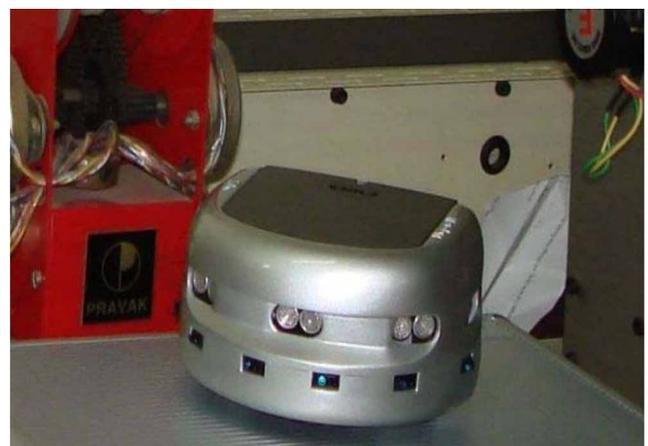
Fig. 11 Khepra-III mobile robot developed by K-team
