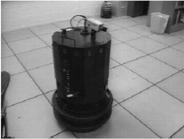
Figure 4: The mobile robot PAVLOV uses discrete-event models to navigate around an indoor office environment.
