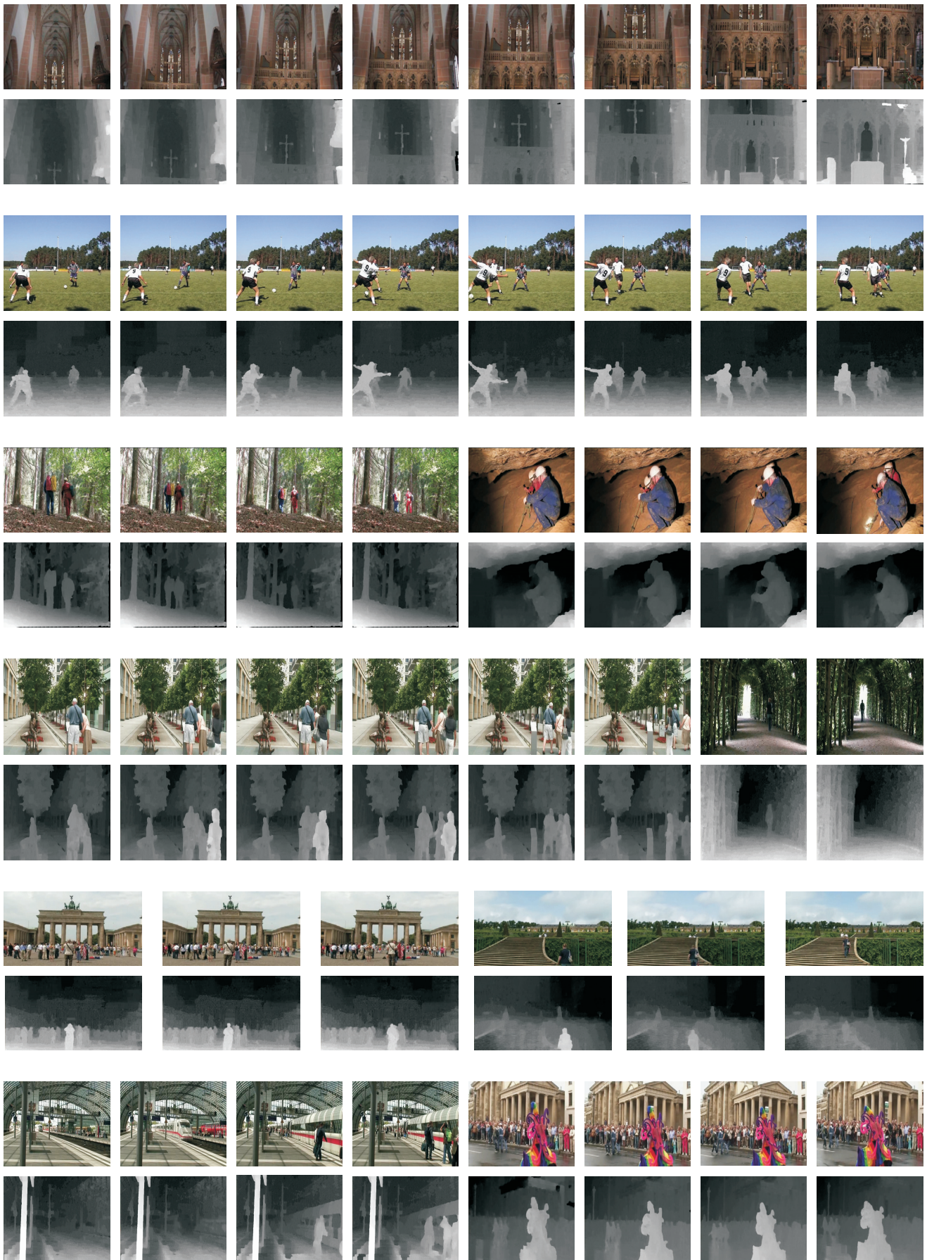
Figure 5. Results of our method. For each sequence, we show the left image of the stereo pair along with the computed temporally smoothed disparity map.
